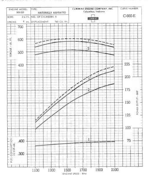
For fire pump applications, the engines are to be applied on the No. 2 performance curve. This is the net torque and horsepower available for fire pump service with all auxiliary equipment connected. The engines are capable of operating on the dotted curve at sea level, 60° F. conditions, which is 15% above the stated net ratings.
